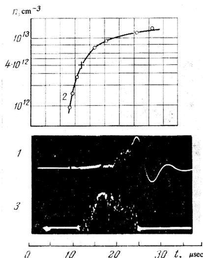
FIG. 4. Plot showing the time variation of the concentration of a plasma with longitudinal current (2) and oscillogram of emission from the plasma at frequency  $3 \times 10^8$  Hz (3). An oscillogram of the longitudinal current is also shown. The period of the current is 7.5  $\mu\text{sec}$ ,  $H = 3$  kOe,  $U_{dir} = 15$  kV.
