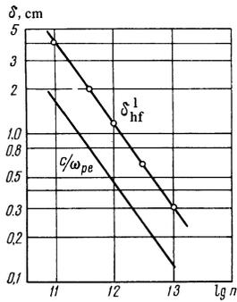
FIG. 3. Dependence of the theoretical thickness  $c/\omega_{pe}$  and the thickness of the experimental skin layer  $\delta_{hf}^l$  on the density of the laminar plasma in the trap.
