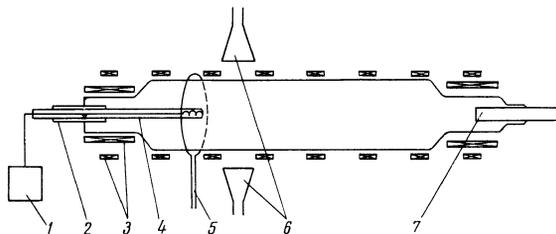
FIG. 1. Diagram of setup: 1 - resonator ( $f_0 = 3 \times 10^8$  Hz) and detector head, 2 - direct-discharge electrode, 3 - magnetic-field coil, 4 - magnetic probe, 5 - transmitting loop, 6 - interferometer antennas, 7 - plasma injector.
