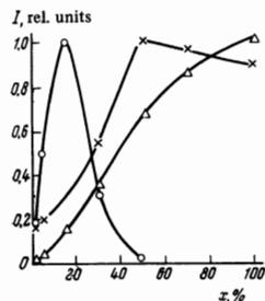
Dependence of the intensity of  $\text{Er}^{3+}$ ,  $\text{Tm}^{3+}$ , and  $\text{Ho}^{3+}$  ions in the crystals: O — [(100 - x)% Y, x% Er]AG, Δ — [(99 - x)% Y, x% Er, 1% Tm]AG, X — [(99 - x)% Y, x% Er, 1% Ho]AG on the concentration of Er at  $T = 77^\circ\text{K}$  (for all the curves the intensities are normalized to unity).
