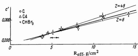
FIG. 2. Measured asymmetry parameter  $c'$  (at meson frequency) vs. target thickness. The double arrow shows the working size of the targets.
