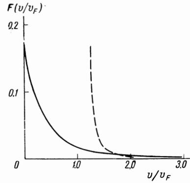
FIG. 2. Dependence of the recombination probability on the velocity of the ion. The dashed curve corresponds to the asymptotic formula (3.15).
