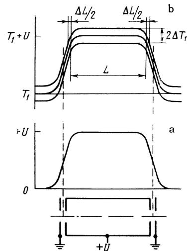
FIG. 2. Potential distribution along collision chamber axis (a) and ion energy at the input to the energy analyzer as a function of the place of formation of the ion from an atom (b).
