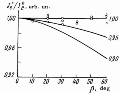
FIG. 5. Ratio of currents of secondary electrons knocked out of a metal plate by fluxes of protons ( $J_e^+$ ) and hydrogen atoms ( $J_e^0$ ), as a function of angle of incidence of the particles on the plate. The smooth curves show the expected behavior of the ratio  $J_e^+ / J_e^0$  for different values of  $\chi$ ; the values of  $\chi$  were taken for  $\varphi = 0^\circ$ .
