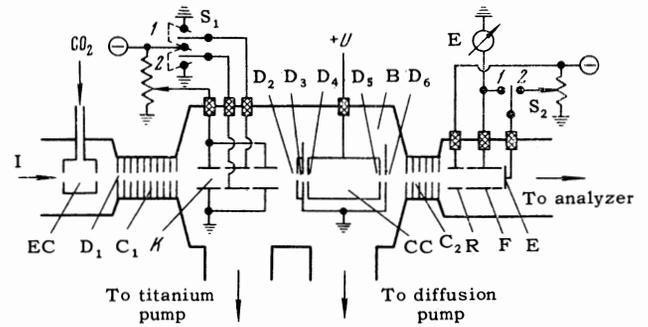
FIG. 1. Diagram of the experimental apparatus: I – primary ion beam, EC – charge-exchange chamber,  $D_1$ – $D_6$  – circular diaphragms,  $C_1$ ,  $C_2$  – vacuum impedances, K – clearing analyzer, CC – collision chamber, B – high vacuum vessel, F – Faraday cup, 3 – movable bottom of Faraday cup, R – reflector,  $S_1$ ,  $S_2$  – switches, E – electrometer.
