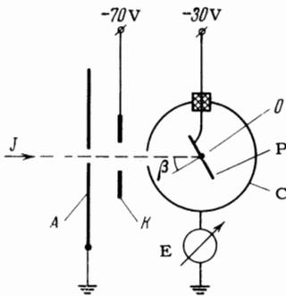
FIG. 4. Diagram of apparatus for determining  $\chi$ : J – atomic, ionic beam, A – aperture diaphragm, P – metallic plate, O – axis of rotation of plate, C – collecting cylinder, K – reflector, E – electrometer.
