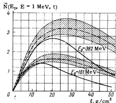
FIG. 5. Cascade curves obtained in the present work (solid lines) and calculated by the method of moments [1] (dashed curves). The shaded region corresponds to the uncertainty in the values of  $E$ , which is  $\pm 0.5 \text{ MeV}$ .
