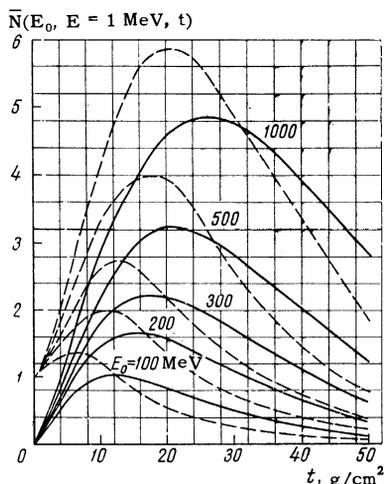
FIG. 3. Cascade curves for showers produced by photons (solid curves) and electrons (dashed curves).
