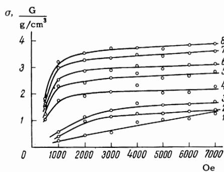
FIG. 2. Isotherms of the specific magnetization of  $U_2Te_3$ : curve 1— $123^\circ K$ , 2— $121^\circ K$ , 3— $119^\circ K$ , 4— $114^\circ K$ , 5— $109^\circ K$ , 6— $103^\circ K$ , 7— $93^\circ K$ , 8— $84^\circ K$ .
