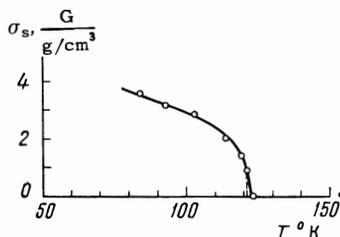
FIG. 3. Temperature dependence of the spontaneous specific magnetization of  $U_2Te_3$ .
