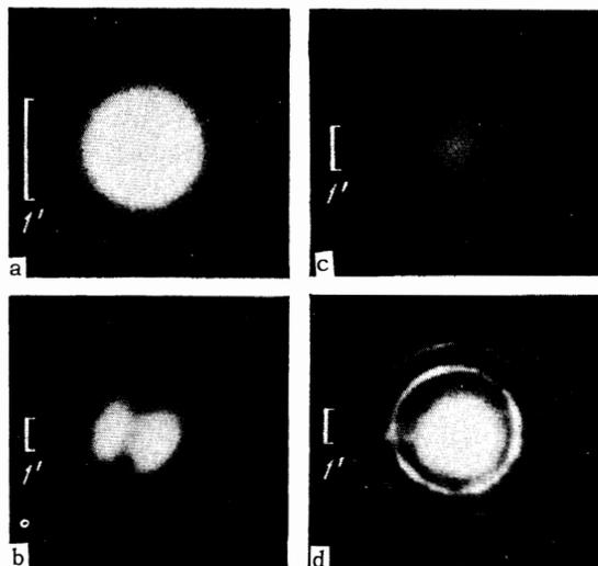
FIG. 1. Photographs of the angular distribution of laser emission. a – neodymium glass; red length  $l = 4.0$  cm, diameter  $D = 0.8$  cm, resonator length  $L = 100$  cm, excess pump power  $n = 20$ . b, c, d –  $\text{CaF}_2:\text{Sm}^{2+}$ ;  $l = 4$  cm,  $D = 0.5$  cm. b –  $L = 60$  cm,  $n \approx 1$ ,  $\text{TEM}_{00}$  mode. c –  $L = 45$  cm,  $n \approx 1$ ,  $\text{TEM}_{01}$  mode. d –  $L = 45$  cm,  $n = 16$ .
