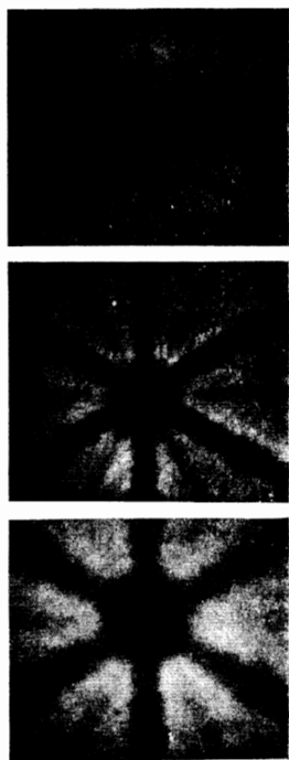
FIG. 2. Proton patterns obtained for molybdenum at incident-proton energies (keV); a – 300, b – 40, and c – 15.
