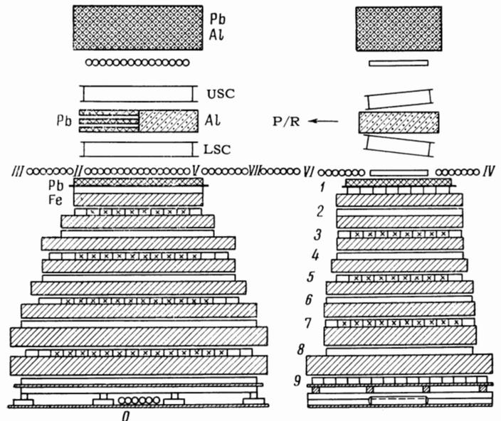
FIG. 1. Schematic diagram of the array in two projections: USC and LSC - upper and lower spark chambers, I - VII and 0 - rows of Geiger-Muller counters, 1 - 9 - rows of ionization chambers of the calorimeter, where the crosses denote chambers connected for coincidence, P/R - spark-chamber photorecorder.
