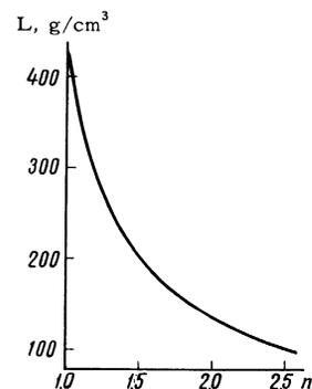
FIG. 2. Plot of absorption path L against the number of particles  $n$  simultaneously incident on the array.
