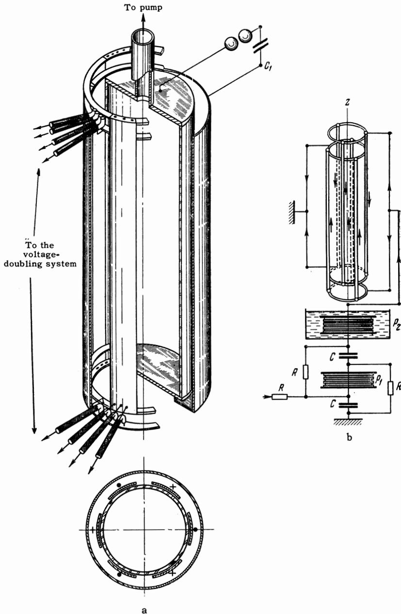
FIG. 1. Schematic diagram of the discharge chamber (a) and supply system for the stabilizing circuit (b).
