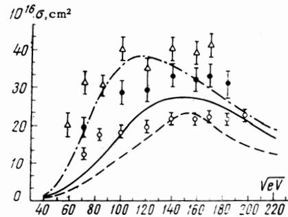
FIG. 2. Cross section for the detachment of an electron from  $H^-$  in Ar, Kr, Xe.  $O, \bullet, \Delta$  – experimental data from [2] for Ar, Kr, and Xe, respectively. The results of the present investigation for  $H^-$  in Ar, Kr, and Xe are represented by dashed, continuous, and chain curves, respectively. The values of the scattering lengths were taken from [5].
