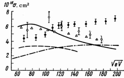
FIG. 1. Cross section for the detachment of an electron from  $H^-$  in He and Ne.  $\Delta$  – experimental data from [3] for He target;  $O, \bullet$  – experimental data from [2] for  $H^-$  in He and Ne, respectively; dashed curve is theoretical, taken from [1] for He target; the continuous and chain curves represent the results of the present investigation for  $H^-$  in He and Ne, respectively. The values of the scattering lengths  $l$  were taken from [4].
