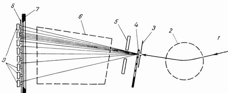
FIG. 1. Experimental arrangement: 1 - ion beam from cyclotron, 2 - magnetic mass analyzer, 3 - diaphragm 1 mm in diameter, 4 - target-scatterer, 5 - sliding channel, 6 - magnetic analyzer, 7 - slit  $0.08 \times 110$  mm, 8 - moveable 2-mm slits, 9 - proportional counters.
