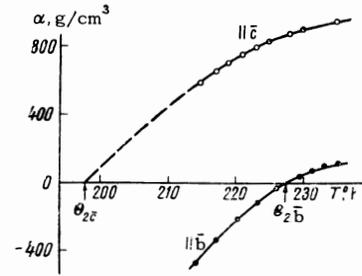
FIG. 3. Temperature dependence of the coefficient  $\alpha$  of a single crystal of terbium along axes  $\bar{b}$  and  $\bar{c}$ .
