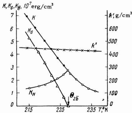
FIG. 4. Temperature dependence of the coefficient  $k'$  and of the constants  $K$ ,  $K_S$ , and  $K_H$  for a single crystal of terbium near the Curie point  $\Theta_2$ .
