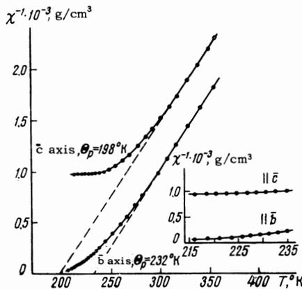
FIG. 5. Temperature dependence of the reciprocal of the paramagnetic susceptibility of a single crystal of terbium along axes  $\bar{b}$  and  $\bar{c}$ .
