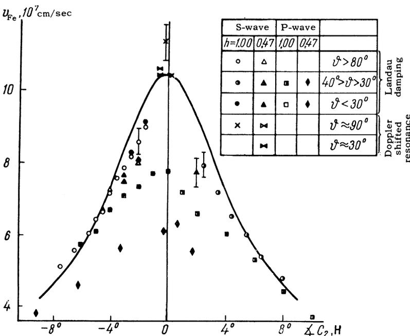
FIG. 6. Determination of the Fermi velocity of electrons. The continuous curve represents the results of calculations based on the Fermi surface model; the error may reach  $\approx 5\%$ . The experimental error is indicated for some of the points.
