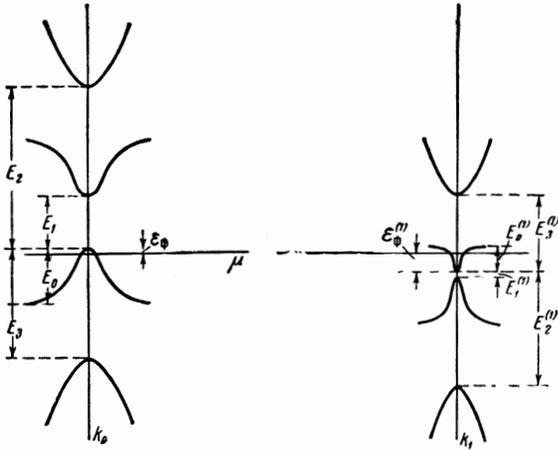
FIG. 2. Diagram of carrier bands in bismuth.
