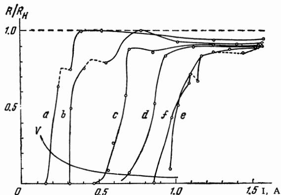
FIG. 2. Dependence of the resistance of a sample on the current at various temperatures ( $T_a > T_b > \dots > T_f$ ).
