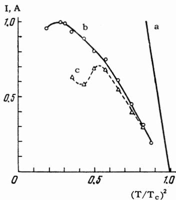
FIG. 3. Temperature dependences of the critical current: a) for bulk metal; b) for a film, according to  $I_c = I(R/R_N = 0.3)$ ; c) for a film, according to  $I_c = I_{V=const}$ .
