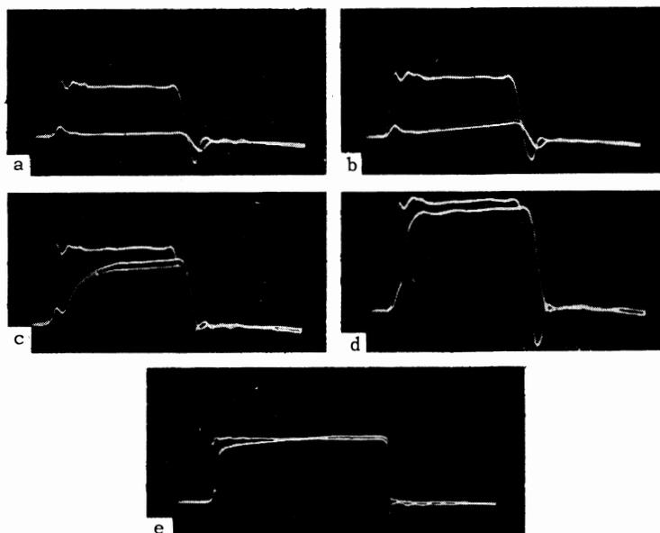
FIG. 1. Current and voltage pulse oscillograms for a sample: a)-d)  $\tau_{\text{pul}} = 0.4 \mu\text{sec}$ ; e)  $\tau_{\text{pul}} = 5.0 \mu\text{sec}$ ;  $I_a = 430 \text{ mA}$ ,  $I_b = 510 \text{ mA}$ ,  $I_c = 630 \text{ mA}$ ,  $I_d = 880 \text{ mA}$ ,  $I_e = 1100 \text{ mA}$ .
