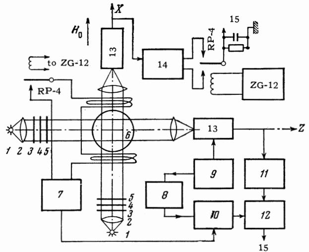
FIG. 2. Block diagram of the experimental setup: 1 - cesium lamp, 2 - lens, 3 - polaroid, 4 - quarter-wave plate, 5 - interference filter, 6 - cell with cesium vapor in argon, 7 - 110 kcs generator, 8 - 50 - 100 kcs converter, 9 - 50 kcs heterodyne, 10 - mixer, 11 - intermediate frequency amplifier of 10 kcs, 12 - synchronous detector, 13 - photomultiplier, 14 - low frequency amplifier, 15 - output.
