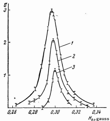
FIG. 6. Broadening of the resonant contour (ac component of the moment) by an alternating field: 1 -  $\omega_x/\Omega = 1.4$ ; 2 -  $\omega_x/\Omega = 0.7$ ; 3 -  $\omega_x/\Omega = 0.35$ .
