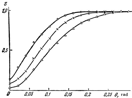
FIG. 3. Dependence of the depth of light modulation on the angle between the constant and alternating fields for three values of the parameter  $\omega_x/\Omega$  (reading upward): 0.2, 0.7, and 1.
