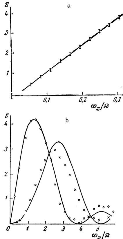
FIG. 4. Dependence of the depth of modulation of light on the amplitude of the alternating field.
