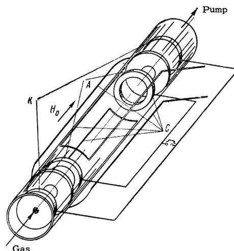
FIG. 1. Drawing of the apparatus: K – cathodes, A – anodes, C – stabilizing current conductors.
