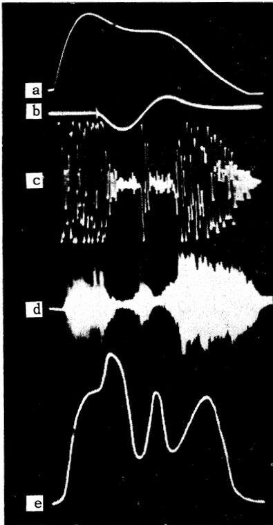
FIG. 2. Oscillograms of discharge processes (pressure  $1 \times 10^{-3}$  mm Hg): a – discharge current, amplitude 100 A, duration 500  $\mu$ sec; b – current in stabilizer conductors; c – alternating component of current in the probe circuit; d – radiation from the discharge, axial component of the electric field; e – direct component of the saturation current in the probe circuit.
