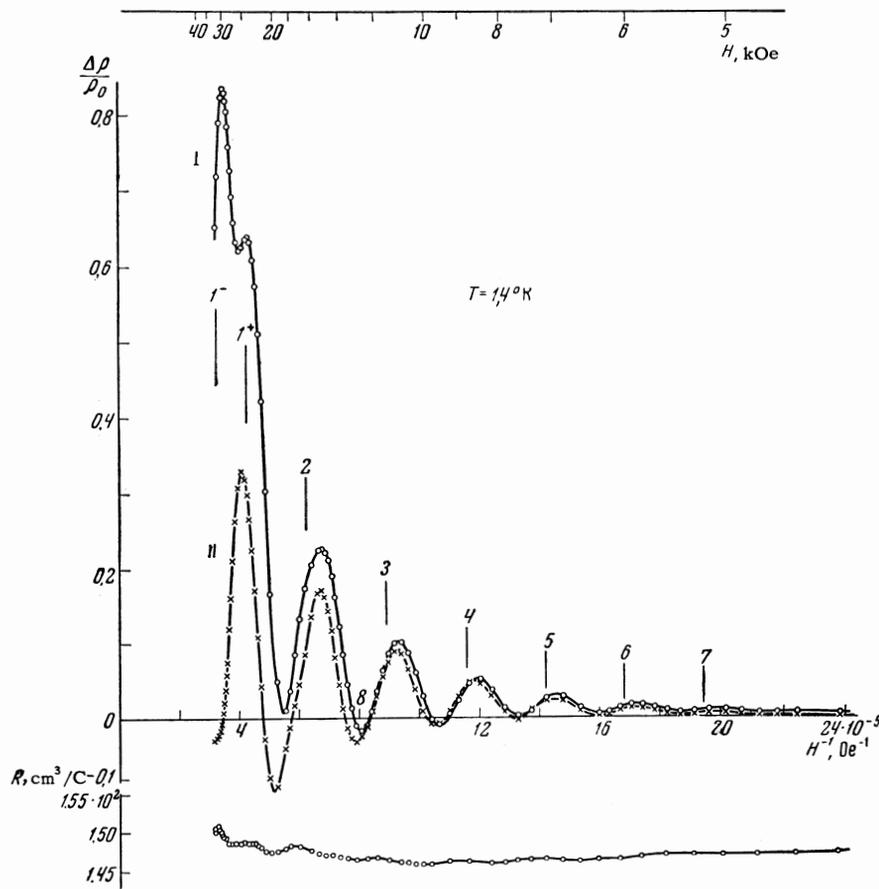
FIG. 2. Experimental curves of the dependence of the transverse ( $\Delta\rho_{\perp}/\rho_0$ ) and longitudinal ( $\Delta\rho_{\parallel}/\rho_0$ ) magnetoresistances of n-type InSb on the magnetic field intensity at  $T = 1.4^\circ\text{K}$ . The lower curve shows the Hall coefficient. The vertical lines with the indices  $1^-$ ,  $1^+$ , 2, ... , have the same meaning as in Fig. 1.
