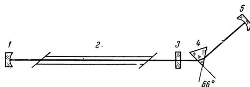
FIG. 3. Diagram of resonator construction for study of the effects of competing transitions.
