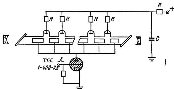
FIG. 2. Schematic diagram of the discharge tube and the exciter. The number of hollow cylinders was 20. Each was 15 cm long, and 1 cm in diameter. The cathode material was stainless steel.
