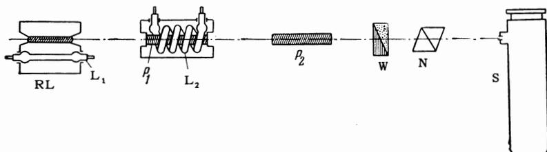
FIG. 1. Optical set-up for observation of dispersion.
