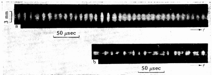
FIG. 2. Distribution of generated radiation at the center of a concentric resonator, photographed with SFR high-speed camera; pump energy 4kJ. a – Crystal at center of resonator, 600 \mu\text{sec} after onset of oscillation; b – crystal shifted 20 cm from center of resonator, 750 \mu\text{sec} after onset of radiation.
