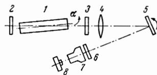
FIG. 1. The optical set-up: 1 – neodymium glass rod of diameter either 8 or 10 mm., length either 67 or 120 mm., and with polished side walls; 2 – dielectrically coated mirror with a reflectivity of 98.5%; 3 – dielectrically coated mirror with reflectivity of 80%; 4 – lens of focal length  $f = 4\text{m}$ ; 5 – rotating mirror; 6 – neutral density filter; 7 – image converter; 8 – camera.
