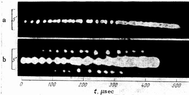
FIG. 2. Time development of the angular distribution in far field pattern. a – axis of the laser rod coincident with that of the cavity to within  $2''$ , b – the axes misaligned by  $40''$ .
