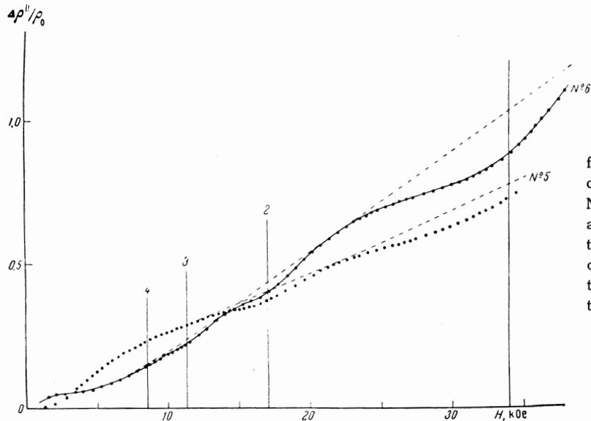
FIG. 2. Longitudinal magnetoresistance curves for two samples of n-type InSb at  $T = 90^\circ\text{K}$ . The carrier densities were:  $1.3 \times 10^{15} \text{ cm}^{-3}$  for sample No. 5;  $4.1 \times 10^{13} \text{ cm}^{-3}$  for sample No. 6 (for details about these samples see [1]). Dashed lines show the postulated magnetoresistance background without the oscillating part. The vertical lines denote those values of the magnetic field which satisfy the resonance condition (1).
