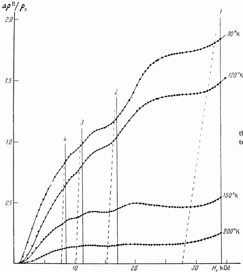
FIG. 1. Longitudinal magnetoresistance curves of the investigated sample of n-type InSb at various temperatures.
