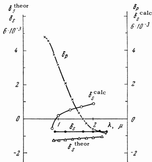
Equatorial Kerr effect in iron for  $\varphi = 45^\circ$ :  $\delta_p$  is the gyroelectric effect,  $\delta_S$  is the gyromagnetic effect,  $\delta_S^{\text{theor}}$  is the gyromagnetic effect calculated using Eq. (1),  $\delta_S^{\text{calc}}$  is the gyromagnetic effect according to [4].
