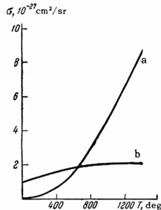
FIG. 1. Dependence of the resonance scattering cross section on the source temperature: a — Ge<sup>75</sup> source,  $\Gamma_\gamma = 4.1 \times 10^{-5}$  eV, b — Sn<sup>123</sup> source,  $\Gamma_\gamma = 6.6 \times 10^{-7}$  eV.
