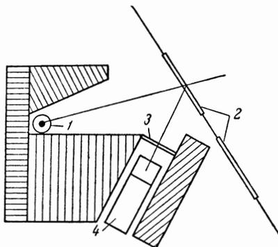
FIG. 2. Diagram of experimental set-up: 1 – electric furnace with source ( $Ge^{75}$  or  $W^{187}$ ), 2 – scatterers, 3 – Pb or Cu filter ( $Sn^{123}$ ), 4 – FÉU-12B photomultiplier with NaI(Tl) crystal.
