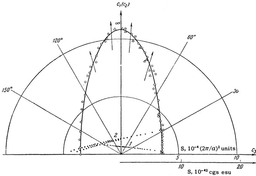
FIG. 1. Anisotropy of the extremal cross sections of the Fermi surface of bismuth obtained for the  $(c_1, c_3)$  plane:  $\circ$  – holes,  $\bullet$  – electrons,  $\Delta$  – holes in the  $(c_2, c_3)$  plane.
