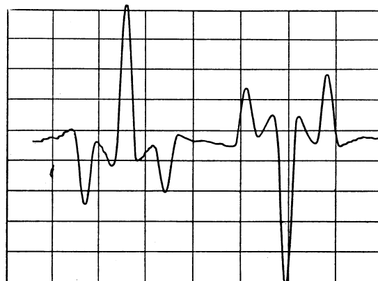
FIG. 3. A record of the dependence of H_0 of the derivative of the real part of the amplitude of the third harmonic for \theta \sim 40^\circ , H_1 = 2 Oe.
