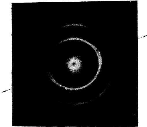
FIG. 8. Cerenkov radiation photograph obtained for a proton beam moving perpendicular to the optical axis of a calcite crystal (outer arcs – ordinary waves, "ellipse" – extraordinary waves, solid ring – radiation from lens, the arrow indicates the direction of the optical axis of the crystal).
