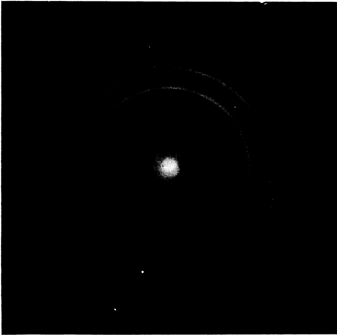
FIG. 3. Cerenkov radiation photograph obtained with the setup of Fig. 1, for a proton beam passing through a calcite slab cut perpendicular to the optical axis (outer ring—extraordinary waves, inner ring—waves from the lens).
