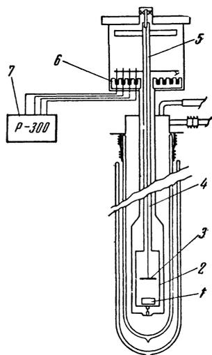
FIG. 2. Diagram of instrument: 1—carbon resistance thermometer, 2—rotating dish, 3—oscillating disk, 4—straightened glass rod, 5—phosphor bronze suspension filament, 6—mercury slip ring contacts, 7—dc potentiometer.
