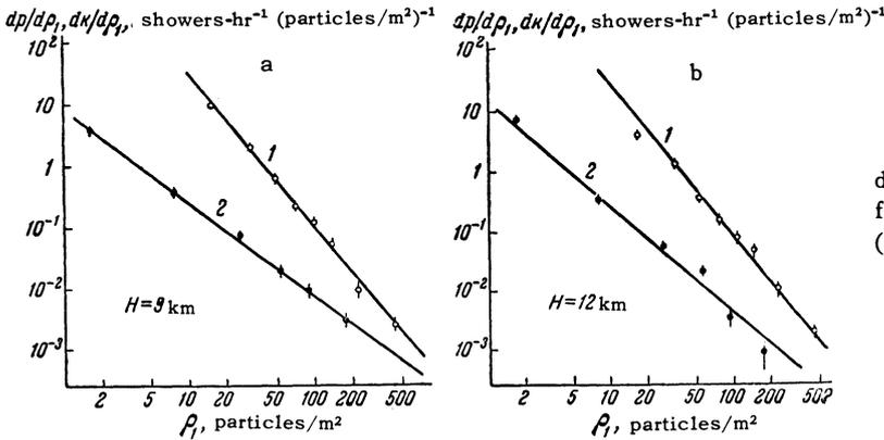
FIG. 2. Density spectra of registered showers  $dp/d\rho$  (curve 1) and  $dk/d\rho_1 (> 7 \times 10^{11} \text{ eV})$  (curve 2) for two altitudes, H = 9 km (311 g/cm<sup>2</sup>) and H = 12 km (197 g/cm<sup>2</sup>).
