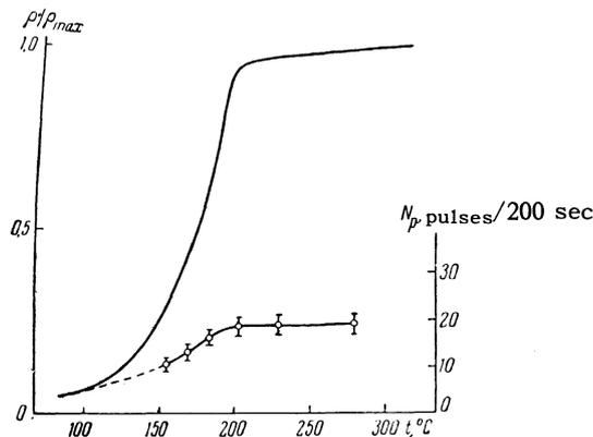
FIG. 2. Density dependence of gaseous source ( $\rho_{\text{max}} = 49$  mg/cm<sup>3</sup>) and experimental value of the resonance effect (points).
