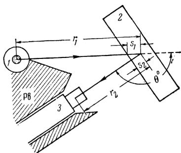
FIG. 1. Experimental set-up (for one channel): 1 – furnace, 2 – scatterer, 3 – detector.
