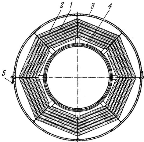
FIG. 5. Section through scattered neutron detector: 1—layer of compound T-1, 2—Plexiglas plate, 3—outer jacket, 4—duraluminum vacuum tube, 5—latch of jacket.
