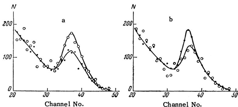
FIG. 1: Spectra of recoil  $\alpha$  particles for coincidences between the helium-chamber pulses and the pulses from the two neutron counters, for opposite directions of the magnetic field of the coil: a—lower counter, b—upper counter; ●—current in the solenoid to the left, ○—current to the right.
