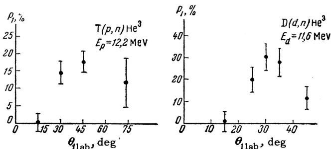
FIG. 2. Angular distributions of neutron polarization.
