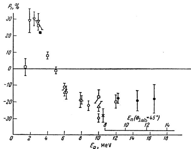
FIG. 3. Energy dependence of neutron polarization in the  $T(p,n)He^3$  reaction:  $\square$  - data of [12],  $\theta_{c.m.s.} = 45^\circ$ ;  $\nabla$  - data of S. E. Darden (private communication),  $\theta_{lab} = 30^\circ$ ;  $\blacksquare$  - [20],  $\theta_{lab} = 33^\circ$ ;  $\triangle$  - [12],  $\theta_{lab} = 40^\circ$ ;  $\circ$  - [11],  $\theta_{lab} = 40^\circ$ ;  $\times$  - [17],  $\theta_{lab} = 40^\circ$ ;  $\bullet$  - present work,  $\theta_{lab} = 45^\circ$ .
