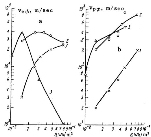
FIG. 2. Dependence of the velocity of azimuthal diffusion of ions and electrons in argon on the value of the field  $B$  for different pressures of the argon.  $I_a = 1.5$  A. Curve 1 -  $p = 41$  N/m<sup>2</sup>, 2 -  $p = 6.3$  N/m<sup>2</sup>, 3 -  $p = 1.55$  N/m<sup>2</sup>.
