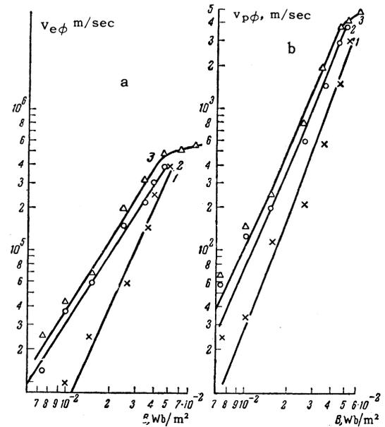
FIG. 1. Dependence of the velocity of azimuthal diffusion of charged particles in a plasma on the value of the applied magnetic field for different values of  $I_a$ . Gas - helium,  $p = 32.5$  N/m<sup>2</sup>. Curve 1 -  $I_a = 0.5$  A, 2 -  $I_a = 1$  A, 3 -  $I_a = 1.5$  A.
