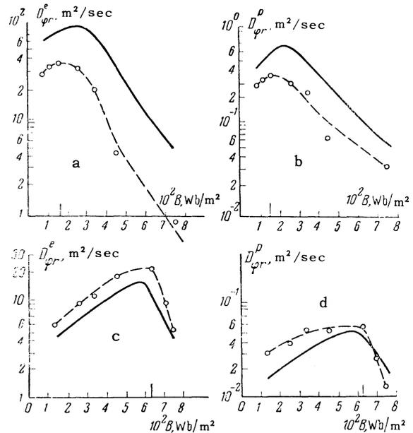
FIG. 4. Coefficients of transverse (Hall) diffusion of electrons and ions according to (12) as functions of the field for two pressures of argon: a, b –  $p = 6.3 \text{ N/m}^2$ ; c, d –  $p = 41 \text{ N/m}^2$ ;  $I_a = 1.5 \text{ A}$ . The dashed curves are experimental, the solid curves are computed by Eqs. (5) and (6).
