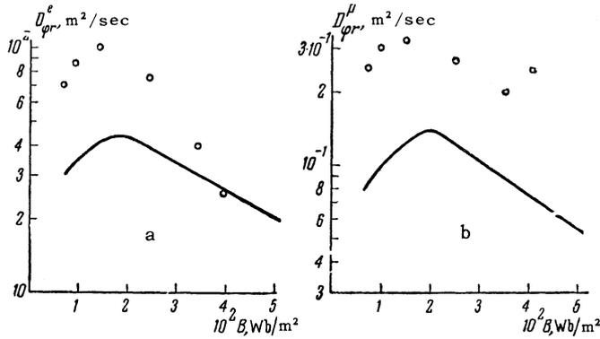
FIG. 5. Coefficient of the Hall diffusion of electrons and ions in helium as functions of the field  $B$ :  $p = 32.5 \text{ N/m}^2$ ,  $I_a = 1 \text{ A}$ . The points are experimental data, the continuous curve is computed.
