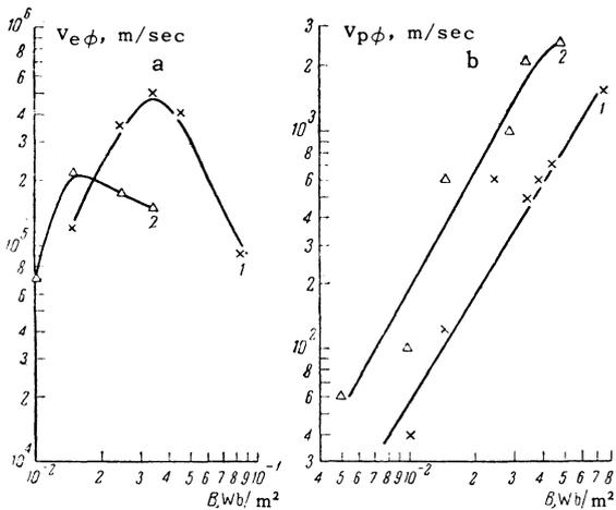
FIG. 3. Dependence of the velocity of azimuthal Hall diffusion of charged particles on the magnetic field in neon,  $I_a = 1.5 \text{ A}$ ; curve 1 –  $p = 10.5 \text{ N/m}^2$ , 2 –  $p = 3.25 \text{ N/m}^2$ .
