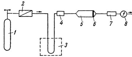
FIG. 1. Schematic drawing of "gas loop." 1 -  $\text{CO}_2$  tank, 2 - reducer, 3 - reactor core, 4 - purifying filter, 5 - accumulating tank, 6 - measuring filter, 7 - exit filter, 8 - flow meter.
