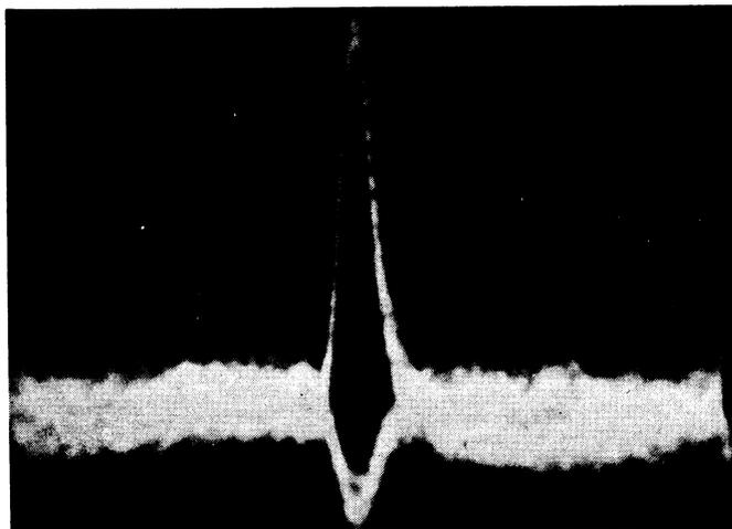
FIG. 1. Photograph of the emission line (positive large pulse) and the absorption line in the beam.
