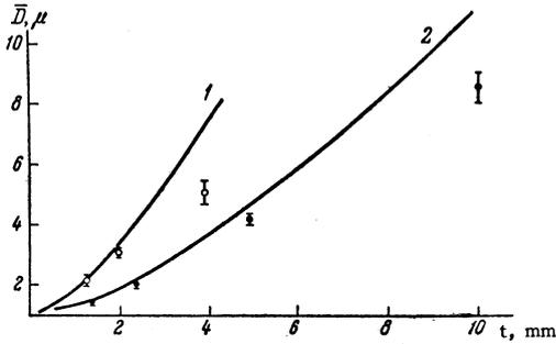
FIG. 5. Variation of the second difference with cell length: 1 and 2—theoretical curves for  $p\beta c$  equal to 1.04 and 2.6 BeV, respectively. The points correspond to experiments at these energies.
