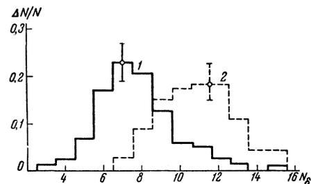
FIG. 1. Distribution of the number of  $\delta$  electrons (per cm); solid line – on tracks of 9 BeV proton (50 tracks), dashed line – 2 BeV protons (60 tracks).
