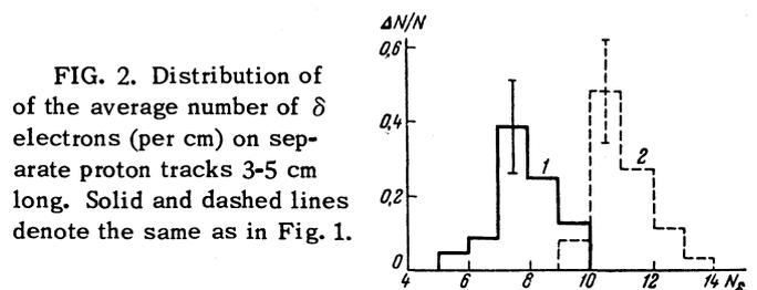
FIG. 2. Distribution of the average number of  $\delta$  electrons (per cm) on separate proton tracks 3-5 cm long. Solid and dashed lines denote the same as in Fig. 1.
