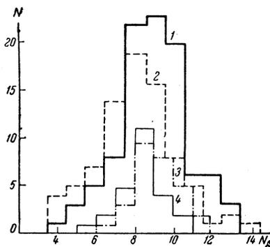
FIG. 3. Distribution of the number of  $\delta$  electrons (per cm) found on particle tracks of: 1, 3–9 BeV protons; 2, 4–secondary particles of  $1.5 \leq p\beta c \leq 2.5$  BeV; 1, 2–as in Fig. 1; 3, 4–as in Fig. 2.
