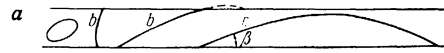
FIG. 1. The trajectories of electrons in a plate in a weak magnetic field parallel to its surface.
