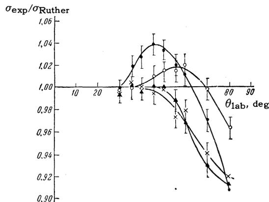
The angular distribution of the ratio of the experimentally measured cross section to the Rutherford cross section for nickel nuclei ( $E_p = 4.2$  MeV):  $\circ$ — $\text{Ni}^{58}$ ,  $\bullet$ — $\text{Ni}^{60}$ ,  $\times$ — $\text{Ni}^{62}$ ,  $\blacktriangle$ — $\text{Ni}^{64}$ .
