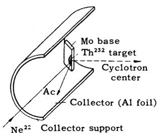
FIG. 3. Device for measurement of the angular distribution of recoil nuclei (in the angular range  $180$  to  $40^\circ$ ).
