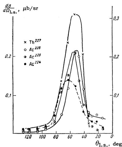
FIG. 4. Differential cross sections for the production of  $\text{Th}^{227}$ ,  $\text{Ac}^{226}$ ,  $\text{Ac}^{225}$ , and  $\text{Ac}^{224}$  in the l.s. for the bombardment of  $\text{Th}^{232}$  by 150-MeV  $\text{Ne}^{22}$  ions ( $\theta$  is the angle of emission of the recoil nucleus).
