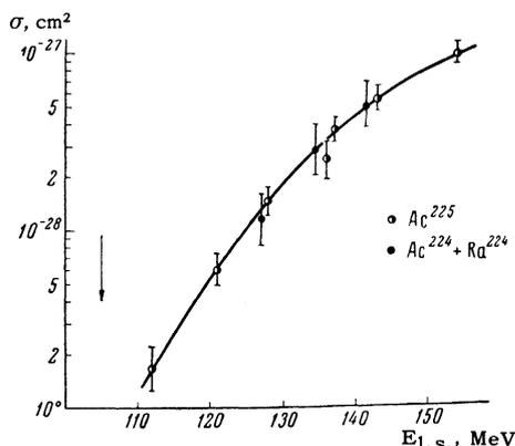
FIG. 2. Energy dependence of the  $\text{Ac}^{225}$  and  $\text{Ac}^{224}$  production cross sections.
