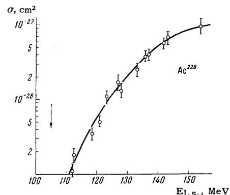
FIG. 1. Cross section for the production of Ac<sup>226</sup> in the bombardment of thorium by Ne<sup>22</sup> ions as a function of the bombarding-particle energy (in the laboratory system). The arrow indicates the Coulomb barrier energy.
