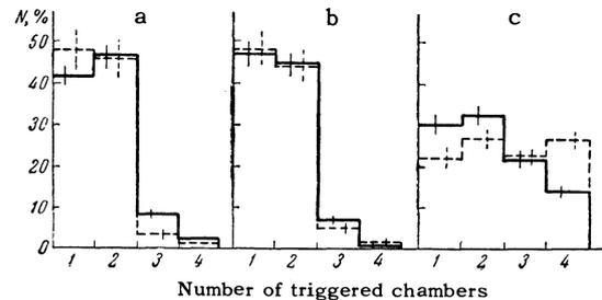
FIG. 2. Distribution of ionization (number of triggered ionization chambers in row III). Abscissa - number of chambers in which ionization exceeded 1/4 of maximum: a) in control experiment, b) in nuclear interactions within apparatus, c) in electron-photon cascades from the atmosphere. Continuous line - measurements at 12 km; dashed line - at 9 km.
