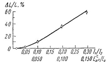
FIG. 3. Mean free path  $L$  for interaction vs. the fraction of energy transferred to  $\pi^0$  mesons.  $I_1/I_3$  is the corresponding ratio of pulse heights in rows I and III.
