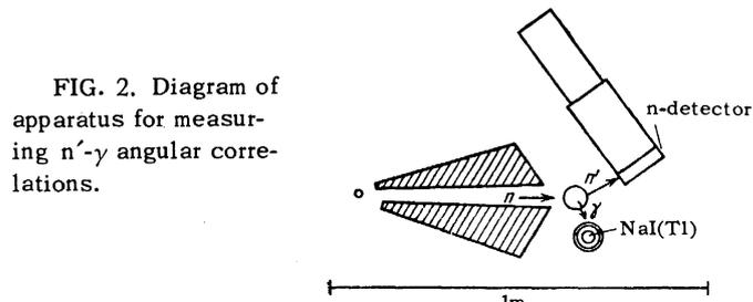
FIG. 2. Diagram of apparatus for measuring  $n'$ - $\gamma$  angular correlations.
