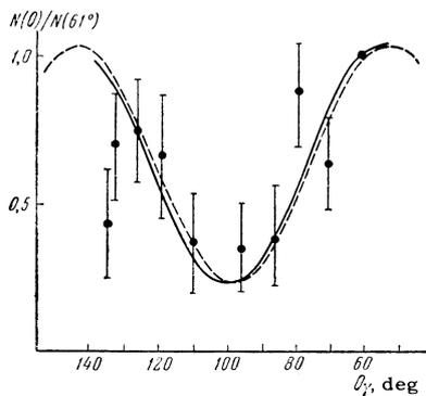
FIG. 4. Angular distribution of 4.4-MeV  $\gamma$ -rays in the reaction  $C^{12}(n, n')C^{12}$  for neutron scattering at the angle  $\vartheta_n = -24^\circ$ . The continuous curve represents the experimental formula (3.1); the dashed curve follows from the theory of direct interactions.<sup>[11]</sup>
