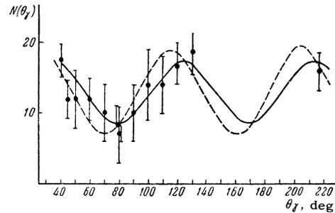
FIG. 5. Angular distribution of 4.4-MeV  $\gamma$ -rays in the reaction  $C^{12}(n, n')C^{12}$  for neutron scattering at the angle  $\vartheta_n = 40^\circ$ . The continuous curve represents the experimental formula (3.1); the dashed curve follows from the theory of direct interactions.<sup>[11]</sup>
