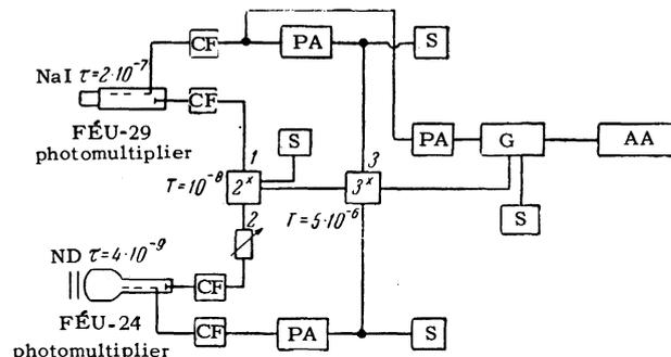
FIG. 3. Block diagram of apparatus for registering  $n'$ - $\gamma$  coincidences. CF – cathode followers, 1 – fast (double) coincidence circuit, 2 – variable delay line, PA – proportional amplifiers (with pulse shaping at output), 3 – triple coincidence circuit, G – gate, AA – amplitude analyzer, S – scaler, ND – neutron detector.
