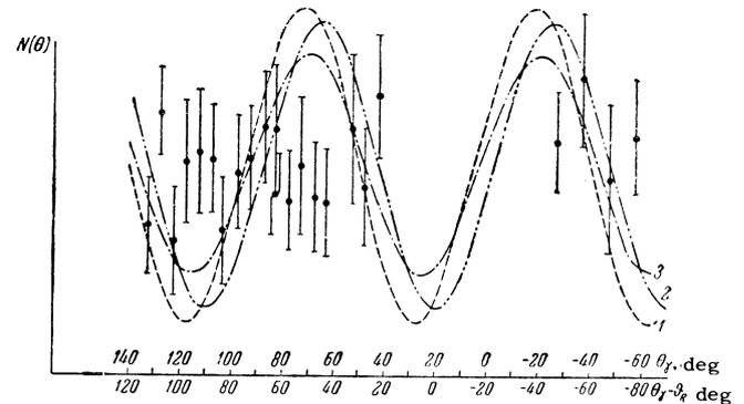
FIG. 6. Angular distribution of 4.4-MeV  $\gamma$ -rays in the reaction  $C^{12}(n, n')C^{12}$  for neutron scattering at the angle  $\vartheta_n = 135^\circ$ . Curve 1 – predicted by direct-interaction theory;<sup>[11]</sup> curves 2 and 3 –  $\gamma$ -ray distribution in the reaction  $C^{12}(p, p')C^{12}$  for  $\vartheta_p = 150^\circ$  and  $110^\circ$ ,<sup>[11]</sup> respectively.  $\gamma$ -ray directions are measured from the direction  $\vartheta_R$  of the recoil nucleus.
