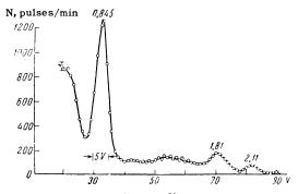
FIG. 3.  $\gamma$  spectrum of the Mn<sup>56</sup> nucleus in the energy range 0.530-2.400 MeV.
