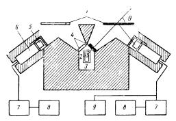
FIG. 2. Experimental setup under the "plane" geometry conditions: 1) scatterers; 2) source; 3) electrical furnace; 4) Fe and Cd absorbers (in the self-absorption experiment); 5) NaI: Tl crystal; 6) FÉU-12B; 7) single-channel pulse analyzer; 8) PS-10 000 scaler; 9) 100-channel pulse analyzer AN-100.
