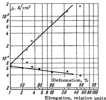
FIG. 2. The dependence of the current densities  $j_{c\parallel}$  (○) and  $j_{c\perp}$  (●) in a field of 23.5 kOe on the degree of deformation and the magnitude of the elongation (Nb + Zr (25%)).
