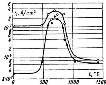
FIG. 4. The variation of  $j_{c||}$  and  $j_{c\perp}$  in a field of 23.5 kOe with annealing temperature  $t$  (alloy Nb + Zr (25%),  $T = 4.2^\circ\text{K}$ ).
