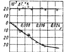
known variation of  $T_K$  with impurity concentration (see the figure, lower curve). The residual resistance ( $r = R_{4.2^\circ K}/R_{20^\circ C}$ ) served as a measure of concentration.
