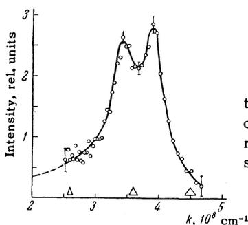
FIG. 3. Intensity of scattered neutrons as a function of wave number;  $\Delta$  is the resolution of the neutron spectrometer.
