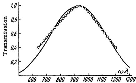
FIG. 1. Comparison of experimentally determined and computed chopper transmission functions.
