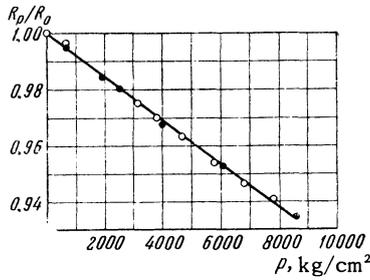
FIG. 1. Effect of pressure on the electric resistance of MnAu<sub>2</sub> at room temperature: ○ – at rising pressure, ● – at decreasing pressure.
