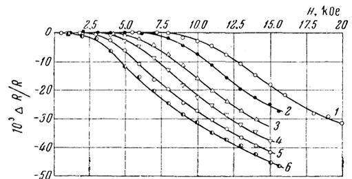
FIG. 4. Dependence of  $\Delta R/R$  on H. Curve 1 – atmospheric pressure; curves 2-6 at pressures (P) 2600, 5400, 7025, 8850, and 10800 kg/cm<sup>2</sup>, respectively.
