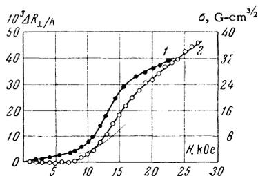
FIG. 3. Dependence of the specific magnetization of MnAu<sub>2</sub> on the magnetic field intensity (1) and dependence of  $\Delta R/R$  on H (2). Room temperature.
