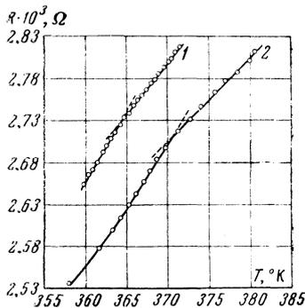
FIG. 2. Temperature dependence of electric resistance: 1 – at atmospheric pressure ( $T_N = 364.6^\circ$ ), 2 – at  $T = 8850$  kg/cm<sup>2</sup> ( $T_N = 370.7^\circ$ ).
