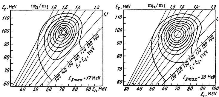
FIG. 2. Contour diagrams for the kinetic energy distribution of fragments for two values of the bremsstrahlung maximum energy. Each contour line corresponds to an increase in the fission probability by 0.1 ( $m_h$  and  $m_l$  are the masses of the heavy and light fragments)
