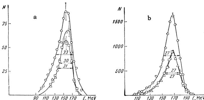
FIG. 3. Spectra of the total kinetic energy of photofission fragments for various bremsstrahlung energies (the numbers indicate the half-widths of the peaks): a—symmetric (in mass) fission, b— asymmetric fission,  $\square$ — $E_{\gamma\max} = 17.5$  MeV,  $\circ$ — $E_{\gamma\max} = 30$  MeV,  $\Delta$ — $E_{\gamma\max} = 50$  MeV.
