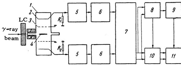
FIG. 1. Block diagram of the experimental arrangement: 1—double ionization chamber, 2—collecting electrodes, 3—grounded shielding grid, 4—high-voltage electrode with thin-film target, 5—preamplifier, 6—amplifier, 7—time-selection circuit, 8—coincidence circuit, 9—intensity-gate circuit, 10—pulse-height memory circuit, 11—cathode-ray tube with two pairs of deflecting plates, LC—lead collimator,  $R_1$  and  $R_2$ —resistances across which the voltage pulse is developed.
